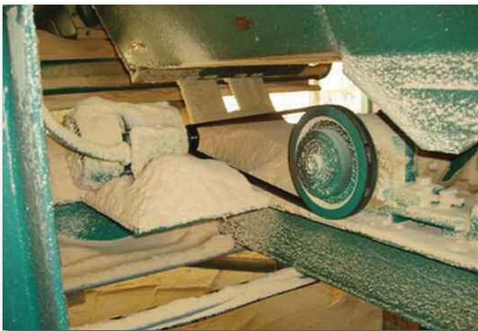
Photo 2: Dust leaks at a material transfer point in a wood planer mill.
