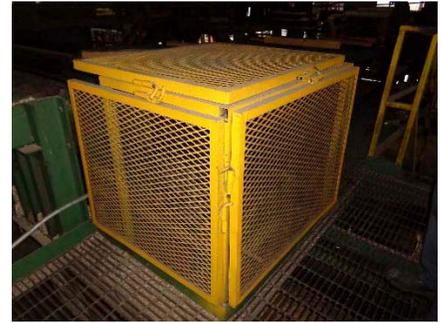
Photo 2: A guarding solution that is hinged for maintenance access and covers the exposed hazard points.
