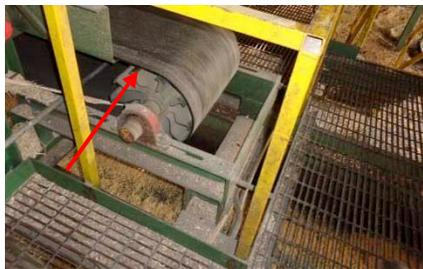
Photo 3: A potential pinch-point hazard from an exposed conveyor belt.
