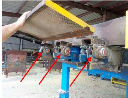
Photo 1: Potential pinch-point hazards from exposed chains on a lumber transfer deck.
