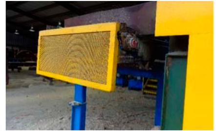
Photo 4: A guarding solution that is hinged for maintenance access and covers the exposed hazard point.
