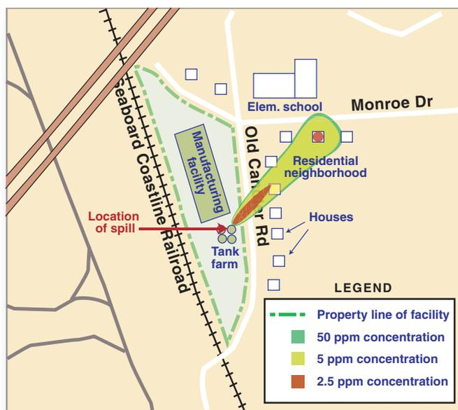
**FIGURE 2.** The dispersion pattern, concentration and impact area of a large hydrochloric acid release (327 lb of 37% solution) at a facility is shown here. This release requires evacuation of the surrounding residents
