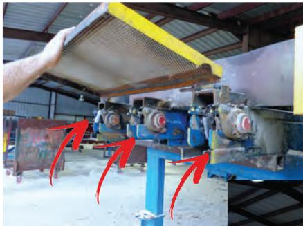
Left: A potential pinch point hazard from exposed chains on a lumber transfer deck
